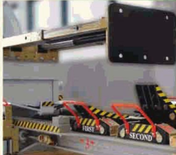
Hydraulic telescopic extended arm for bundle insertion
