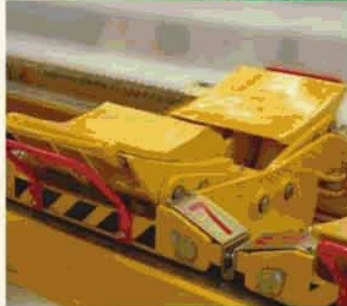
Hydraulic telescopic extended arm for bundle insertion
